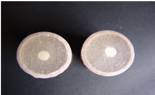
Figure 4. PVC cylinders positioned for filling with acrylic resin.
