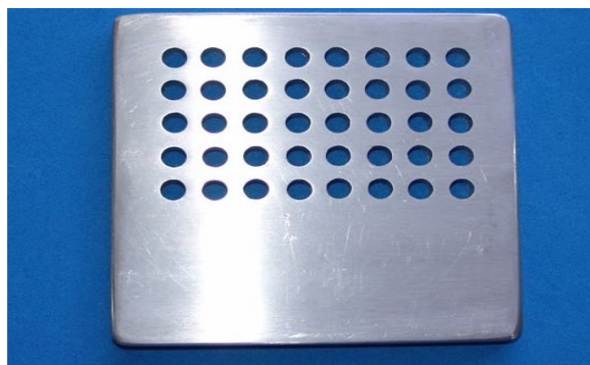
Figure 1. Matrix for construction of the ceramic discs.
