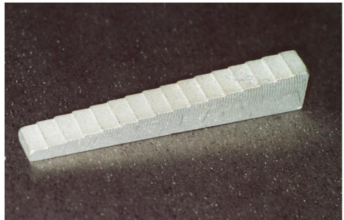
Figure 1. Aluminum step-wedge.
