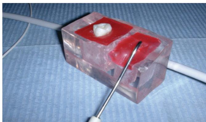
Figure 1. Tooth fixed on an acrylic block and strap for closing the circuit.
