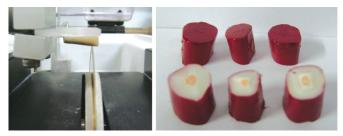
Figure 1. A) Sample in the cutter; B) Waterproofing of test specimens.
