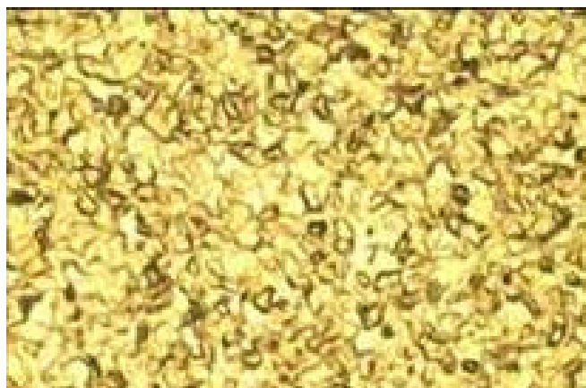
Figure 4 . Ti pellets - Crystallographic granular structure SEM 200x.
